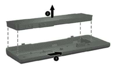
Removing a battery pack from the travel battery caddy
